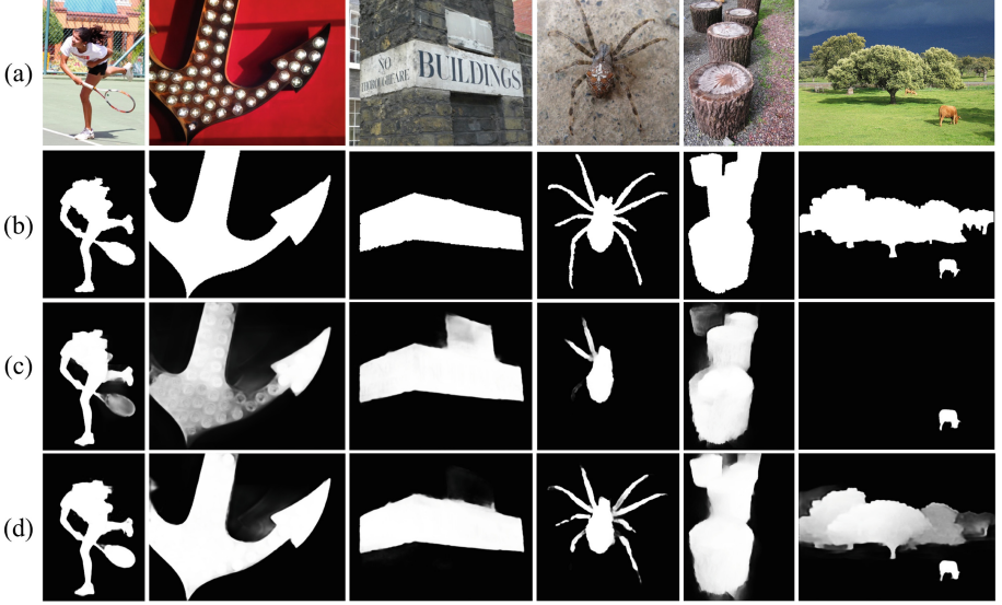
Fig. 3. The effectiveness of GPM. (a) Input images. (b) Ground Truth. (c) Results of our method w/o GPM. (d) Results of our method. We can see that without the GPM, the proposed method will suffer from semantic dilution, interference from non-salient objects, and inaccurate localization of objects.
